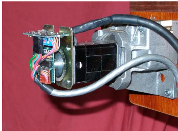
Figure 4.3 - Small DC servo motor with encoder (left) and gearbox
