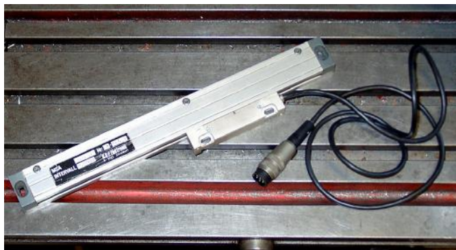
Figure 4.15 - Glass scale encoder (awaiting installation)
