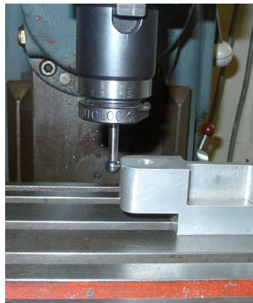
Figure 7.12 - Edge-finder in use on a mill
